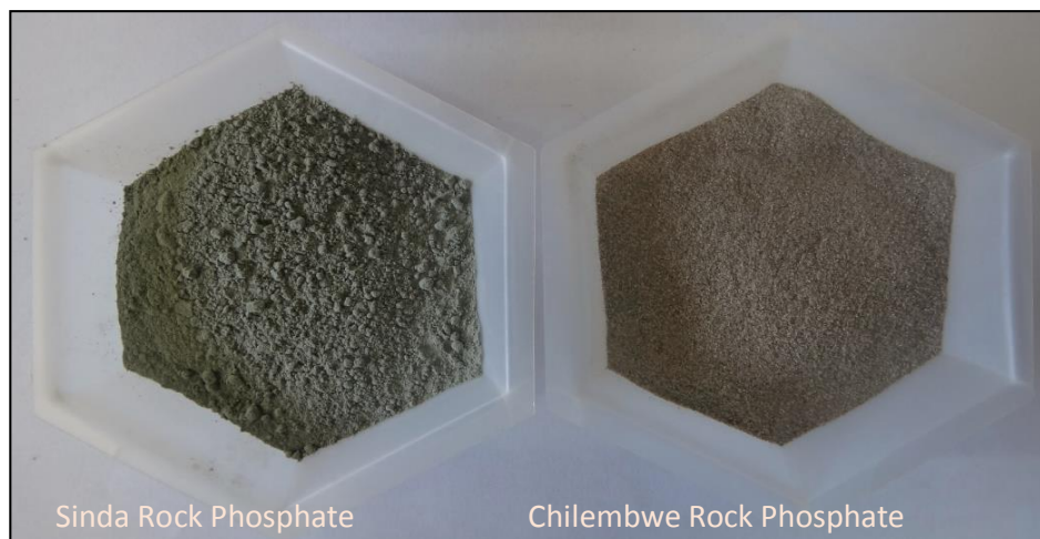
Figure 1. Crushed Sinda and Chilembwe rock phosphates.
